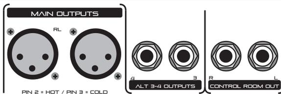
Fig. 2.14: Uscite Main mix, Alt 3-4 e control room
